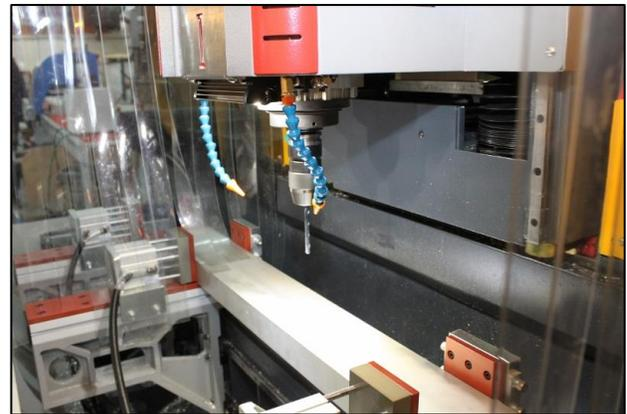
Left: Gamco Corporation's newly acquired CNC Machining Center significantly speeds fabrication of linear aluminum components. Right: Drilling, notching and routing along 3 axes are enabled directly through computer-controlled programming, speeding production, minimizing waste and enhancing quality.
